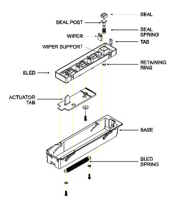
Figure 5-13. Service Station, Exploded View.
